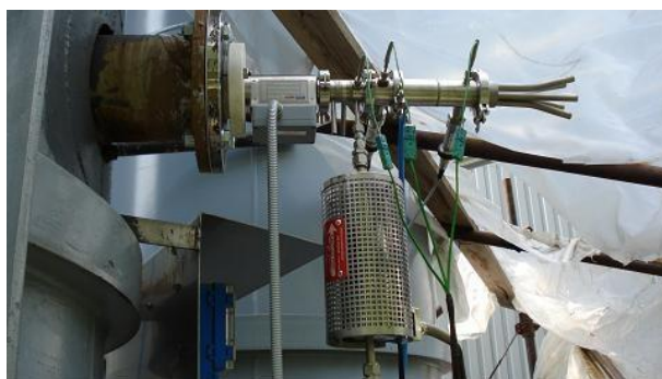
UF particulate sampling system in conveyed streams
