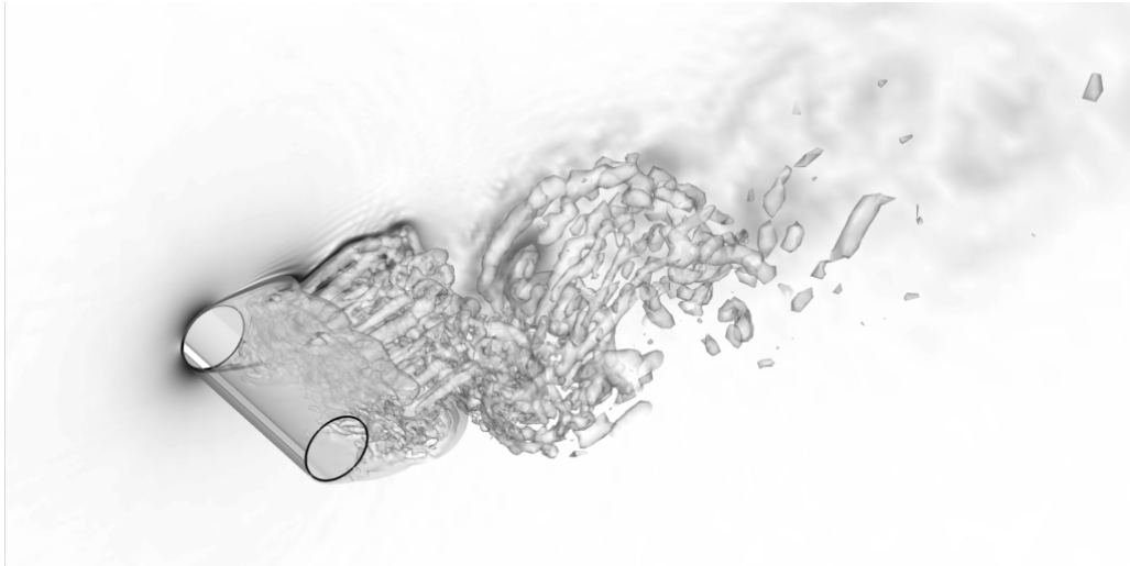
Figure 1: Vortical structures visualized by the Q-criterion, with the numerical Schlieren field displayed on the vertical plane.
