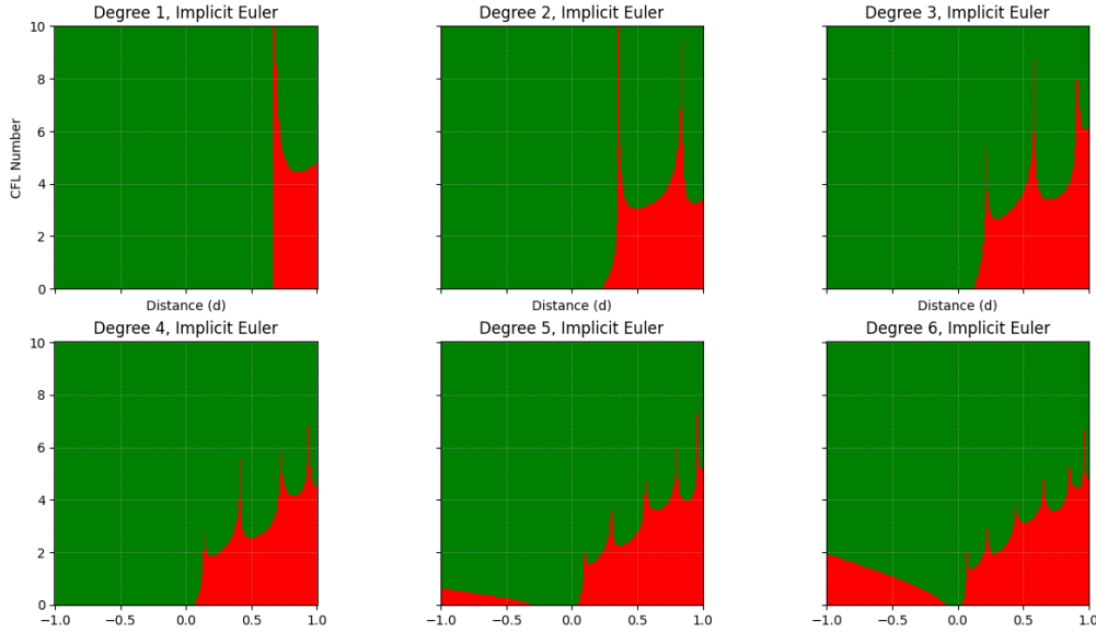
Figure 11: Stability region: ROD- L^2 correction of the homogeneous Dirichlet condition for the implicit discontinuous Galerkin method and \text{CFL} \in [0, 10] . Green areas are stable, while red areas are unstable.
