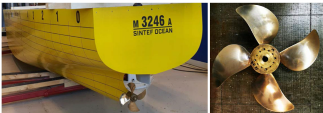
Figure 2: SOCB-1 hull and the CP propeller geometry for physical model tests ([16]).
