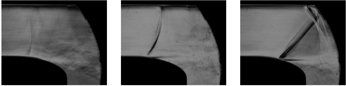
(a) Cat. (A): intermittent near-normal shock motion. (b) Cat. (B): oscillating \lambda -shock. (c) Cat. (C): extended recompression shock system.
