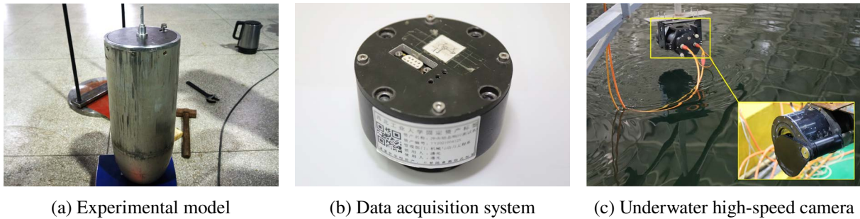
Figure 3: Experimental model and test apparatus.
