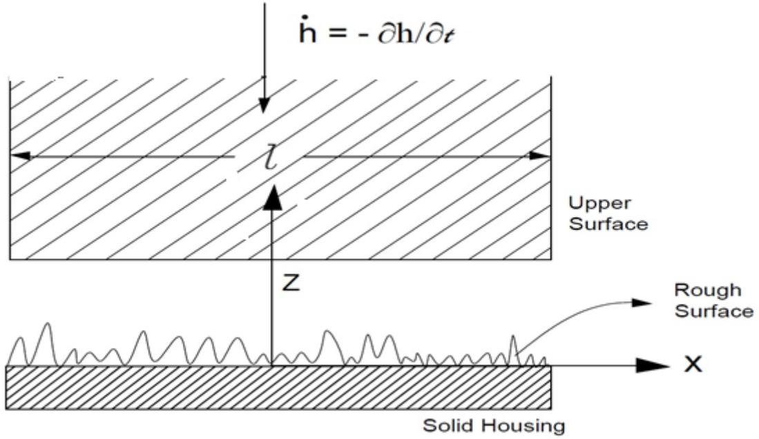
**Figure – I Configuration of the bearing system**
