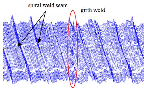
(a) Weak magnetic signal near the girth weld
