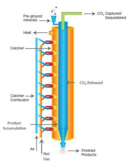
Figure 3: Diagram of the LEILAC Direct separation calciner
