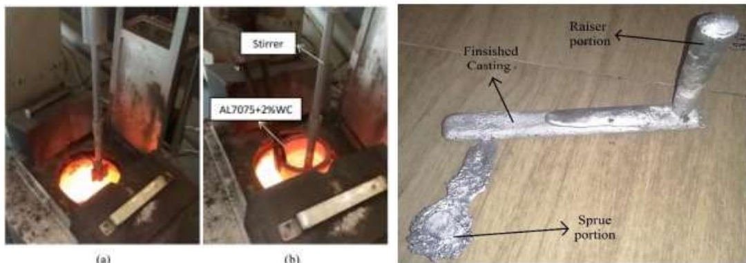
Fig: 4. (a) Stir casting setup at specific temperature (b) mixing of molten metal of Al7075 with Tungsten carbide (WC)
