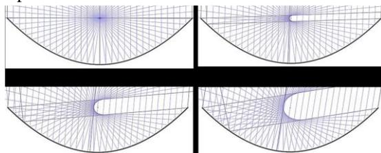
**Fig. 3** Parabolic concentrator scheme at different angular positions
