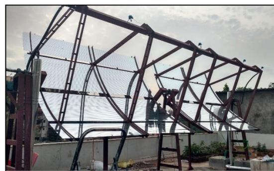
**Fig.1** Parabolic trough solar collector at MVP
