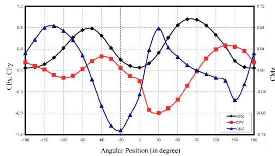
**Fig. 4** Angular position of shape coefficients and aerodynamic coefficients of external PTCs
