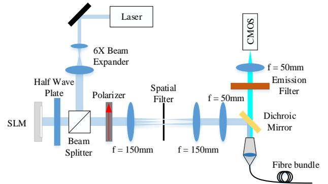
**Fig. 1** Schematic of the proposed imaging system. A grid pattern is produced by a SLM and projected onto a sample via an imaging fibre bundle.
