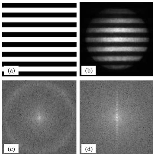
**Fig. 2** (a) Pattern with a rectangular grating to be displayed on the SLM. (b) Image of a thin uniform fluorescent plane illuminated with the pattern in (a). (c) Corresponding Fourier transform of the image in (b). (d) Centre origin of the Fourier transform in (c).
