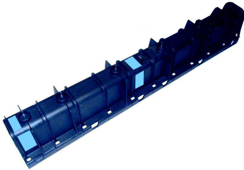
Fig. 10. A photograph of the investigated part with the marked samples cut for microtoming and structure investigation
