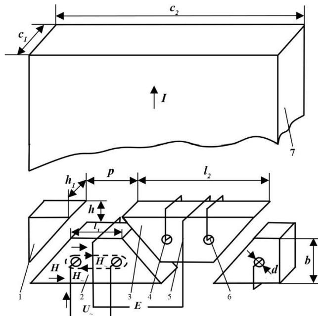
Fig. 1. Part of information non-contact magneto-modulation converter of large direct currents
