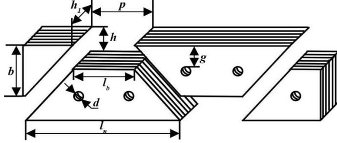
Fig. 3. Geometrical dimensions of the MNT magnetic circuit
