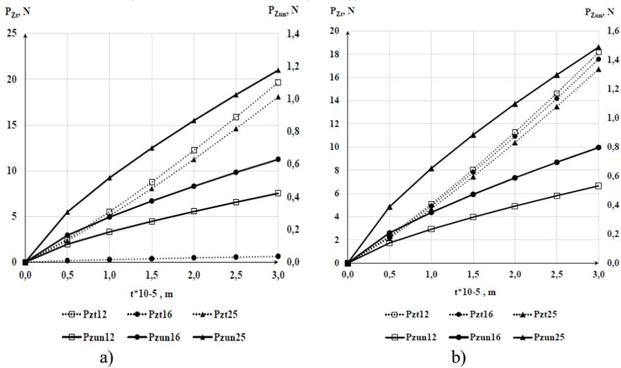
**Fig. 2:** The values of the unit and total cutting forces  $P_z$  during grinding with CBN circles of structure No. 6 - a) and structure No. 40 - b). Modes :  $V_w = 30$  m/s;  $V_{sp} = 0.166$  m/s;  $S = 0.002$  m / v. (LO250/160 C10 100% (Nz25))
