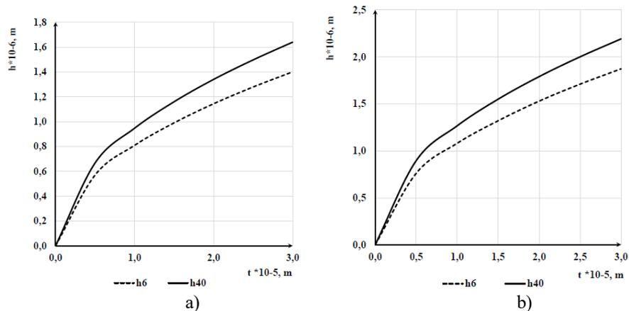
**Fig. 5.** The magnitude of the deepening of grain into material I when grinding CBN with wheels (LO250/160 100% (Nz25)) of structure No. 6 and structure No. 40. Modes  $V_w = 30$  m/s;  $V_{sp} = 0.166$  m/s;  $S = 0.002$  m / rev. Grain a) Nz = 12; b) Nz = 25
