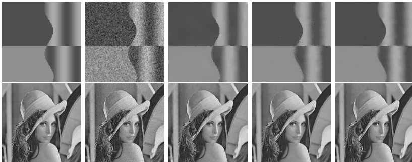
Fig. 3. Denoising results of synthetic and Lena images. The first column: (top) original image synthetic , (bottom) original image Lena . The second column: (top) noisy image for synthetic image, \sigma_n = 20 , (bottom) Lena image, \sigma_n = 10 . The third-fifth columns: denoised images using ALLT, NLTV, and NLABH methods.
