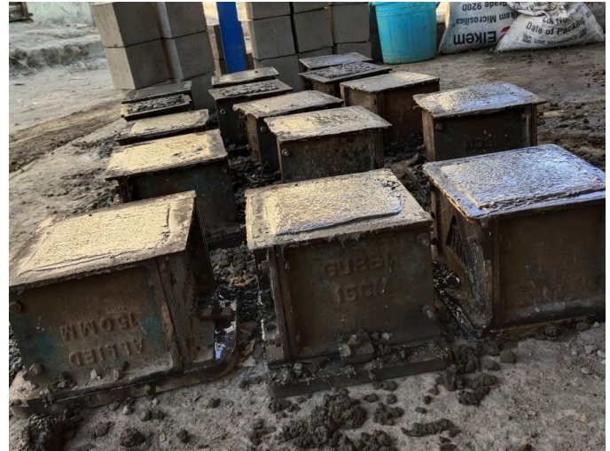
FIG-1: CASTING OF CUBES
