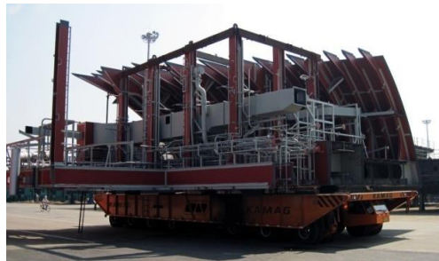
Figure 1. Transport ship block by a flatcar
