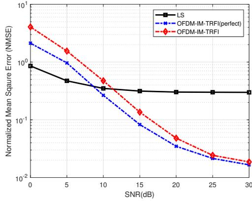
Fig. 2. NMSE performance for M-TFRI and LS scheme with OFDM-IM in VTV-UC environment
