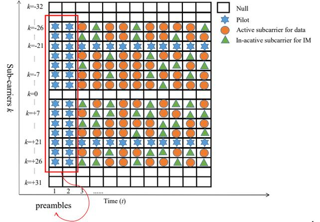
Fig. 1. IEEE 802.11p subcarriers arrangement
