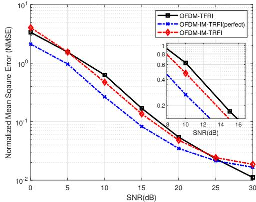
Fig. 3. NMSE performance for M-TFRI and TFRI scheme with OFDM-IM and OFDM in VTV-UC environment
