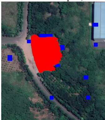
Fig. 9 Detecting sample distribution (Red is landslide test sample, blue is background test sample)
