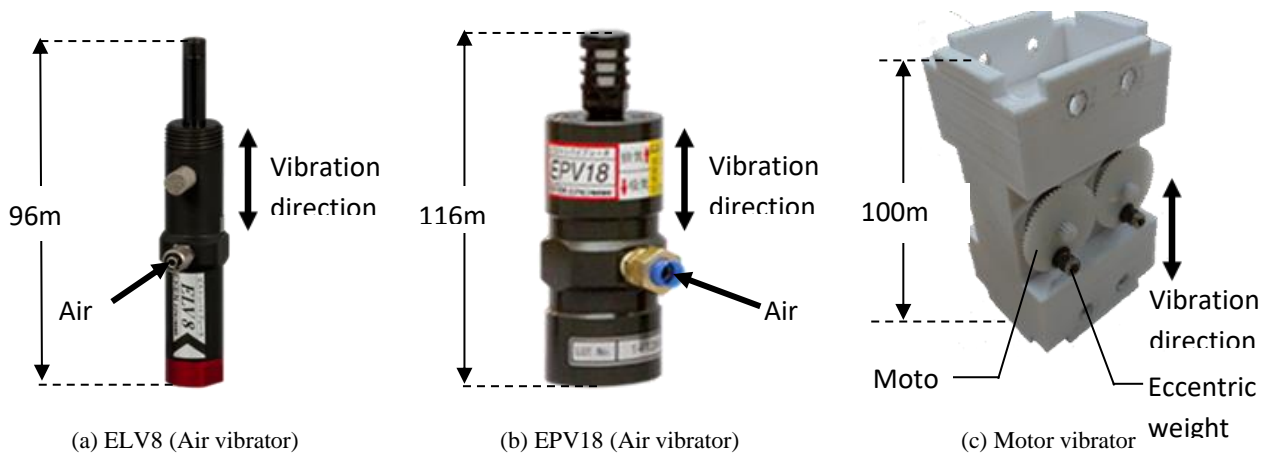
Fig. 2. Air vibrators used in self-weight loading experiment
