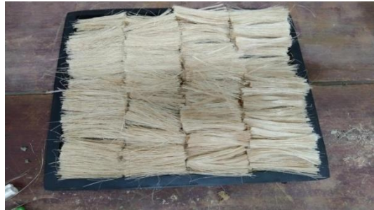
Figure 1. Banana fibres of 60 mm length (Optimized length)
