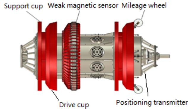
**Fig. 2. Structure diagram of the weak magnetic internal detection device of the pipeline**
