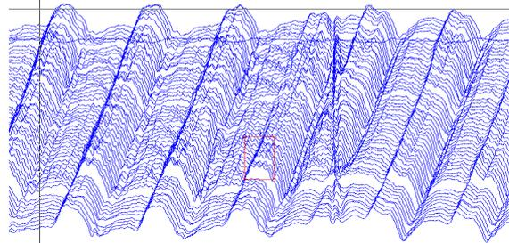
(b) Characteristics of stress concentration signal caused by indentation at the end of the steel pipe
