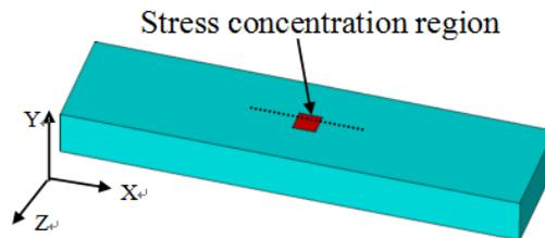
**Fig. 3 Steel plate magnetostatic model of the stress concentration.**
