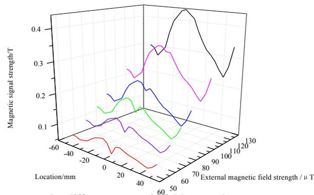
**Fig. 5 Magnetics curve under different magnetic field strengths**
