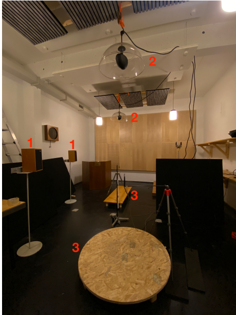
Fig. 1: Test setup showing three of the sound systems. (1) HiFi loudspeakers, (2) parabolic loudspeakers and (3) the platforms with attached transducers. Also seen in the figure are HBK microphones. Only one was used for calibration. The placement seen in the picture does not represent the actual placement for the tests.
