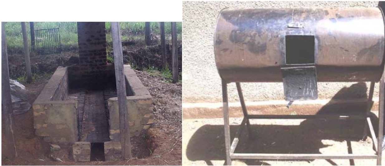
Figure 2: Brick built kiln used for carbonizing bagasse and a cylindrical mixer
