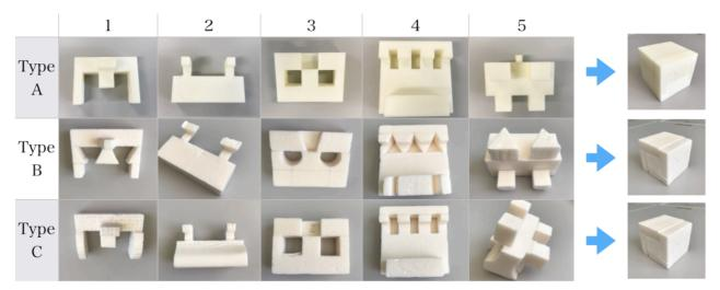
Figure 1: Various parts of joint member in Type A, Type B, and Type C.
