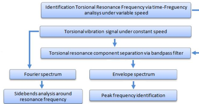
Figure 7. Spectrum analysis flow diagram
