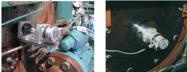
Figure 3. a) Example of a torsion encoder [5], b) Example of a torsigraph [6]
