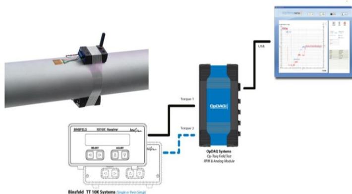
Figure 4. Torsional vibration test kit from Binsfeld Engineering [7]
