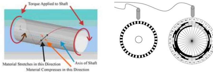
Figure 2. a) Example of shaft exposed to torsion, b) Basic principle of encoder [2]
