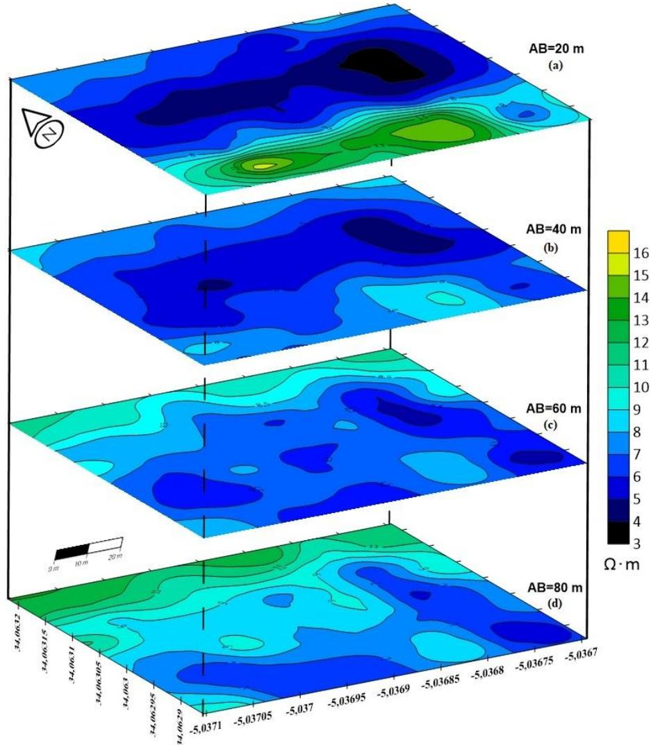
**Fig. 6.** Iso- resistivity maps for AB = 20, AB = 40, AB = 60, AB = 80.
