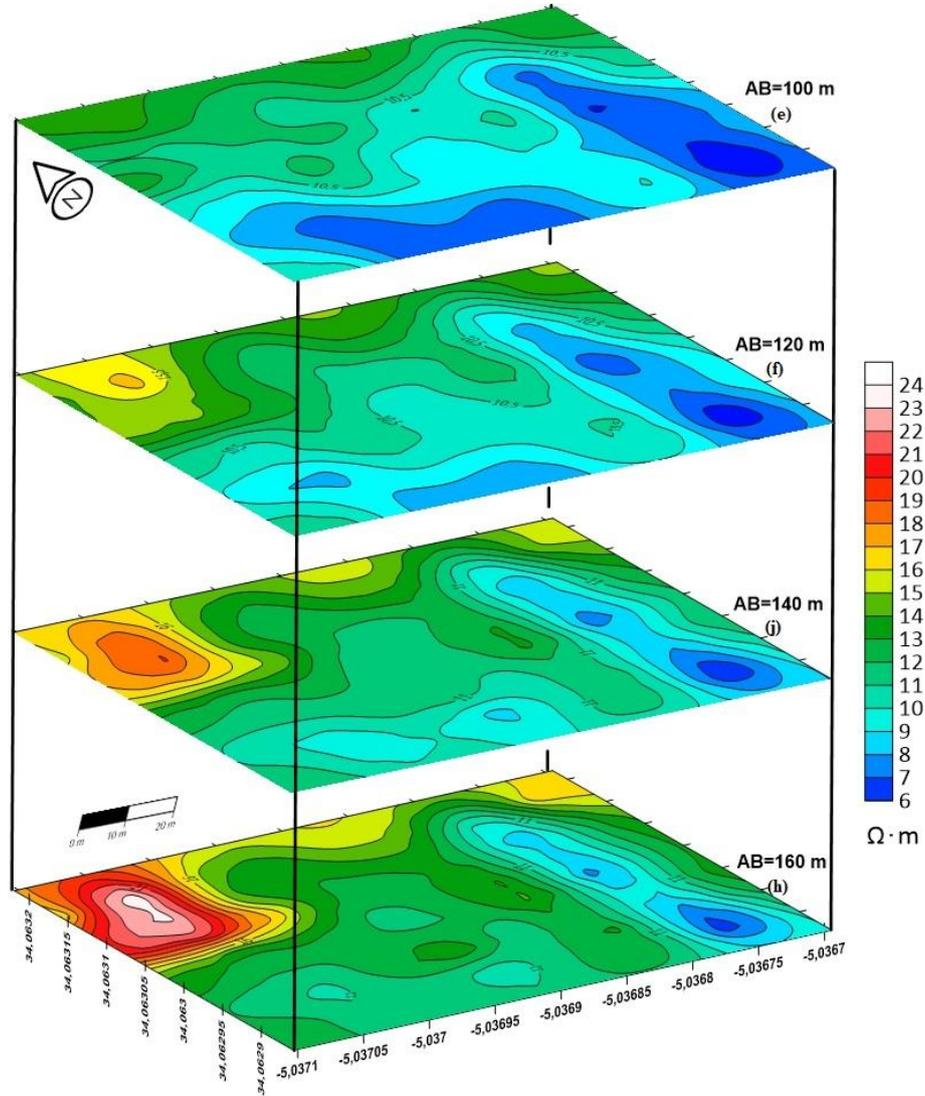
**Fig. 7.** Iso-resistivity maps for AB = 100, AB = 120, AB = 140, AB = 160.
