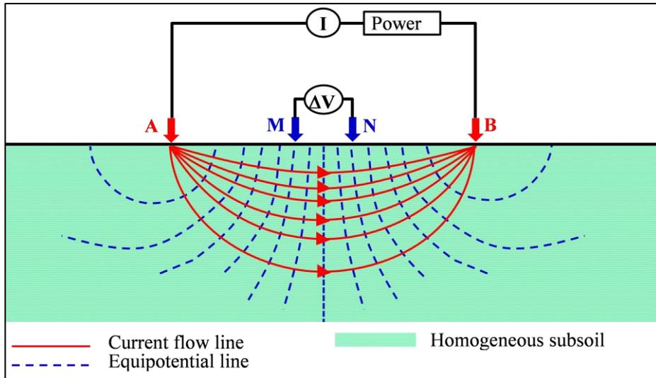
**Fig. 4.** Wenner-Schlumberger array ( $MN=a$ ;  $AM = n \times a$ ) and distribution of electric field underneath in homogeneous medium.
