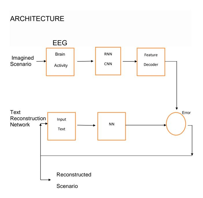
Figure 1 : Architecture for Reconstructing Scenario.
