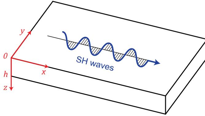
**Fig. 1.** SH guided waves in an orthotropic layer
