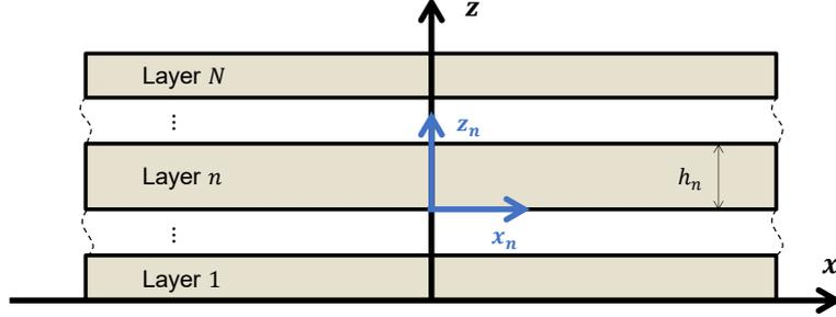
Fig. 2. Laminated composite plate
