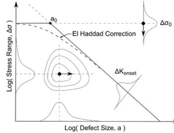
Figure 3 Kitagawa diagram and propagation threshold
