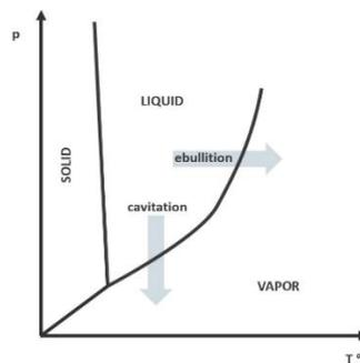
Figure 8 Water state diagram
