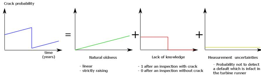
Figure 4 Components of degradation
