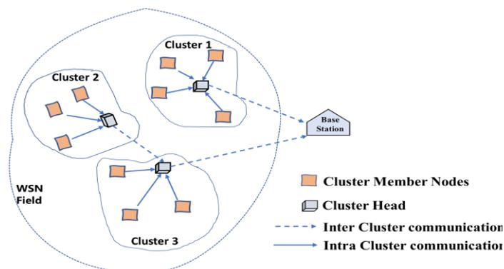
Fig. 2: Architectural design of cluster based HetWSN.
