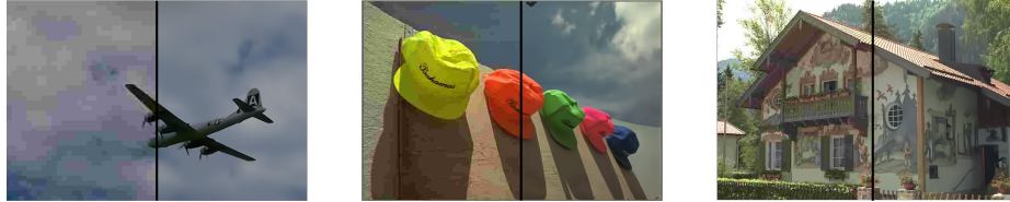
Fig. 1. Visual comparisons. The left side of the image is the JPEG compressed image and the right side is the image that has been reconstructed by our method.
