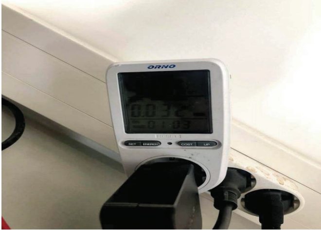
Fig. 8 Example of measuring consumer energy ( laptop ) in an hour
