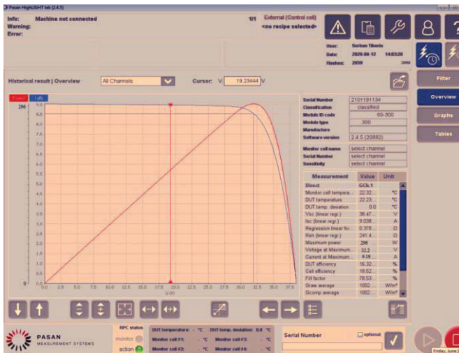
Fig. 12 300W crystalline photovoltaic panel measurement
