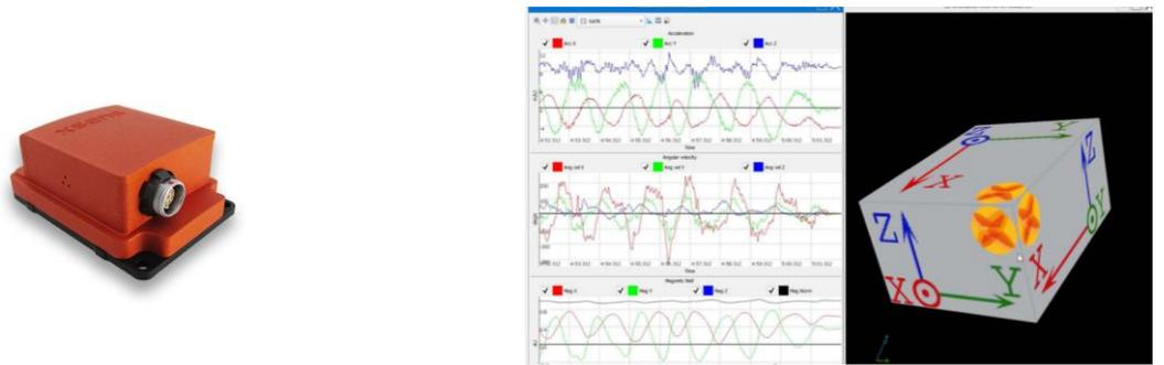
Fig.8. Inertial Measurement Unit (IMU)
