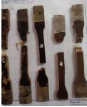
Figure 6: Tensile test specimen after test
