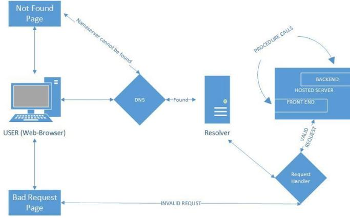
**Figure 3: functional block diagram of the working solution**
