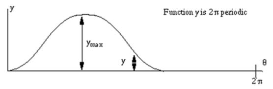
The lift function is a displacement. Its first derivative can be used to compute the velocity, v, and the acceleration, a, of the follower. If w is the angular velocity in radians per second of the camshaft, then v = w y' and a = w2 y''. There is a third derivative quantity the "jerk" which is the time derivative of acceleration, j = w3 y'''. The jerk is the time rate of change of acceleration. The larger its value, the more likely the cam is to create undesirable vibrations in the engine.
