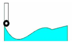
The edge of the flat plate cam can be shaped to give different vertical movements of the cam follower. Flat plate cams or linear cams as they are often called are used frequently in machines which carry out the same repetitive movements.
