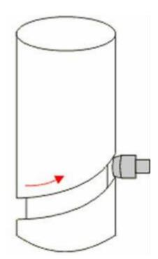
These unusual cams are normally composed of a cylinder which has a groove cut out of its surface and it is in this that the follower runs up and down. This type of cam can be seen in some old clock mechanisms and still in modern sewing machines. Machines that perform repetitive movements may use a cylinder cam profile.
