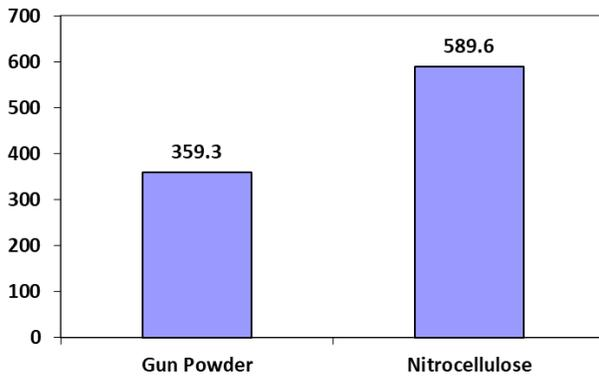
Fig. 8: Mean of Muzzle Velocity (m/s)
