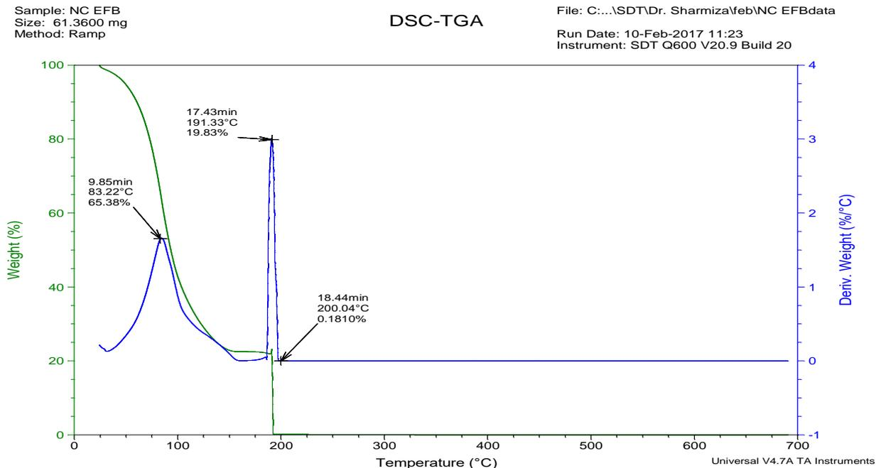
Fig. 12: DSC-TGA for EFB Nitrocellulose
