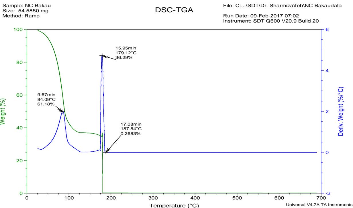
Fig. 11: DSC-TGA for Rhizophora Nitrocellulose
