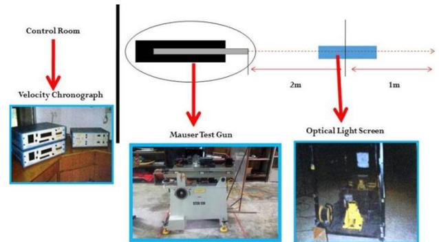
Fig. 3: STRIDE's Experiment Layout
