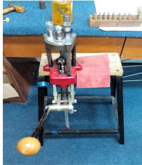
Fig. 6: Reloading Press
