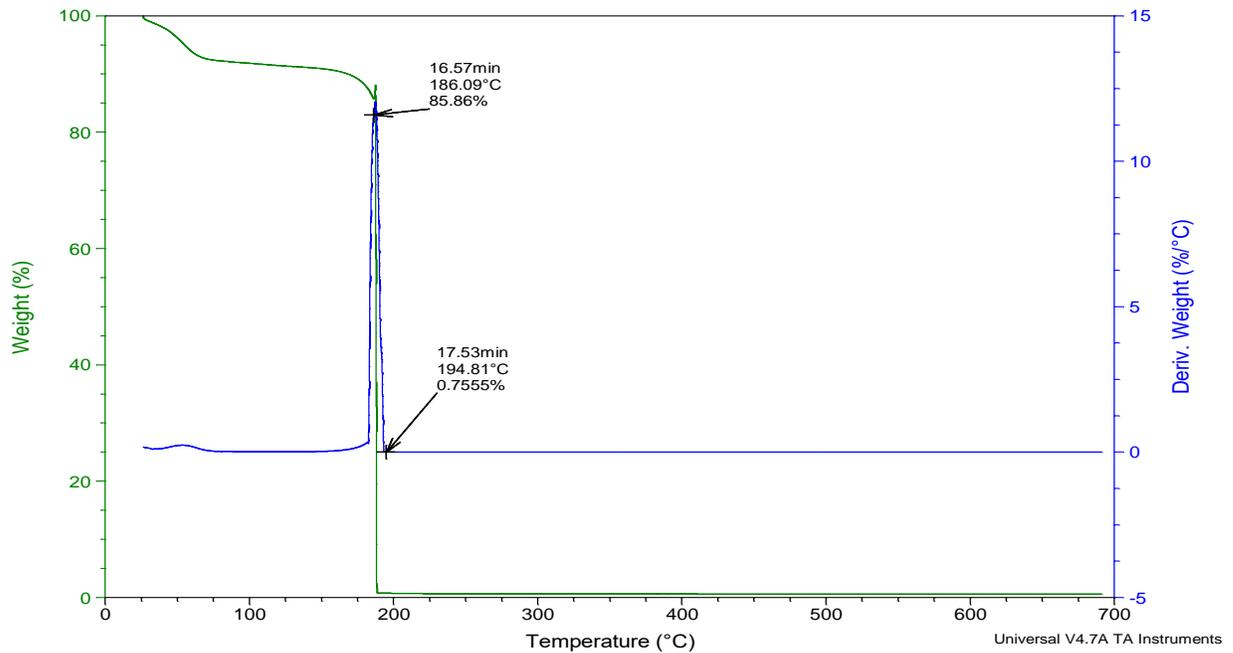
Fig. 13: DSC-TGA for Kenaf Nitrocellulose
