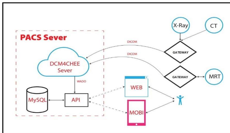
Fig. 1. The core DICOM PACS architecture
