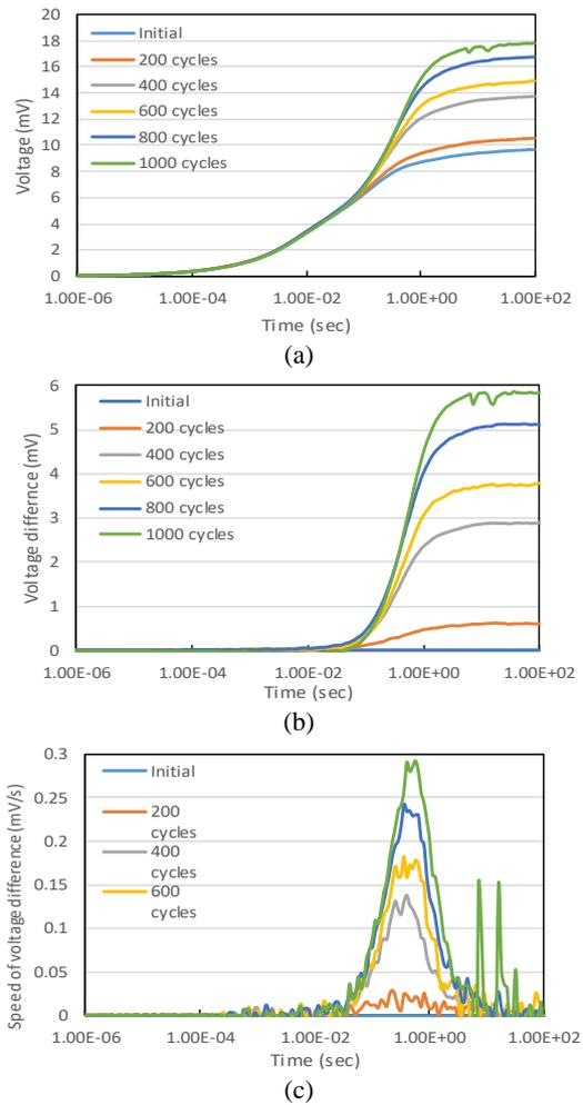
Fig.3 Transient voltage (a), normalized transient voltage (b), and sensitivity function (c) of a LED package.
