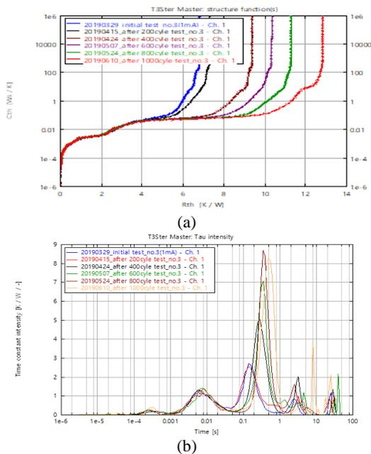
Fig.2. Structure function analysis of a LED package: (a) thermal capacitance–thermal resistance relationship (b) and thermal time constant.
