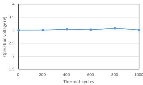
Fig. 1. Static operation voltage of a LED package during thermal shock test.
