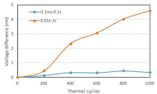
Fig.4. Voltage difference based on 2-point measurement of a LED package with respect to thermal shock test.
