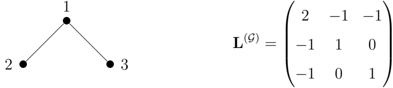
Fig. 3.3: Left: Example of an FL network \mathcal{G} with three nodes i = 1, 2, 3 . Right: Laplacian matrix \mathbf{L}^{(\mathcal{G})} \in \mathbb{R}^{3 \times 3} of \mathcal{G} .
