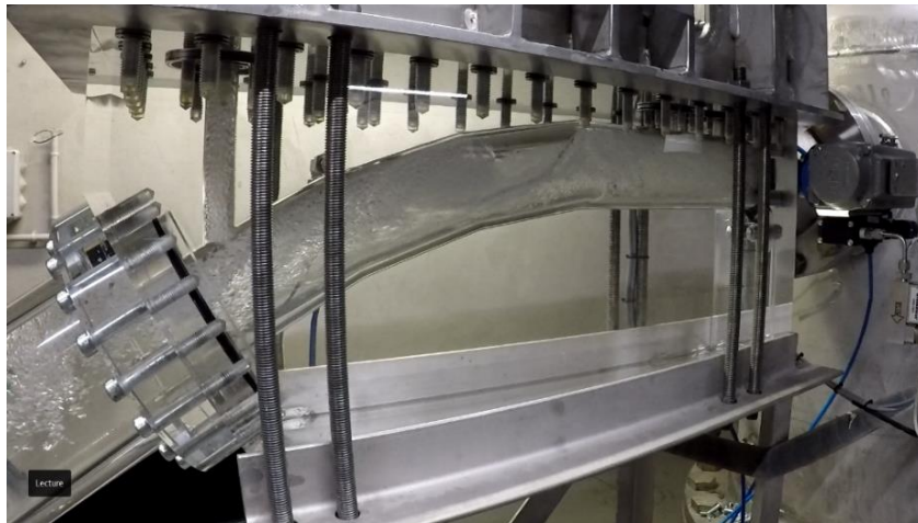
Figure 8 Picture of two-phase air-water flow on the small-scale experiment
