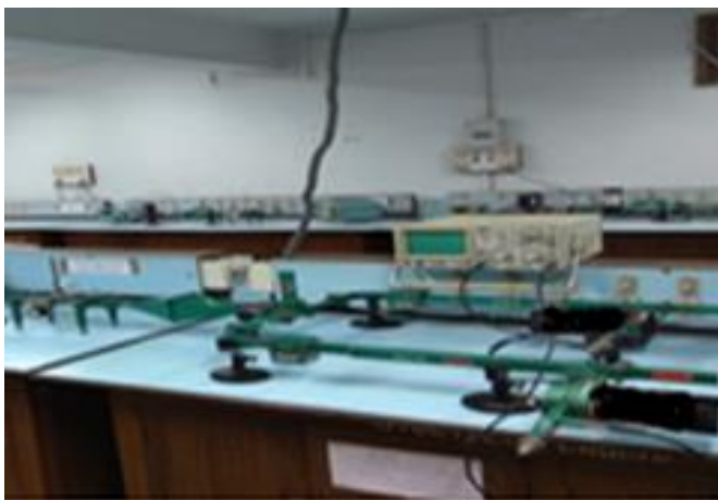
Fig.15. Setup of klystron characteristics using external modulation
