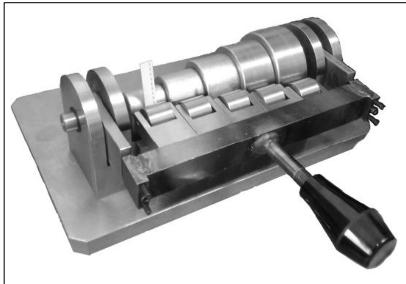
Figure 2. The experimental device for determination of the SBP angle (Slota et al. , 2013).
