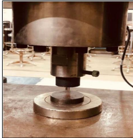
Figure 11. The compression test apparatus.
