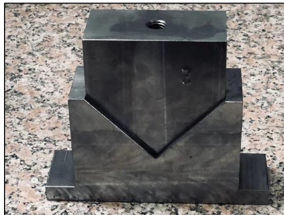
Figure 10. The kind of the mold profile when the V-mold is completely applied.
