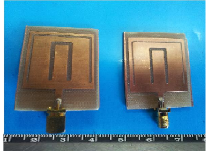
Fig. 8: Fabricated antennas with 50 \Omega SMS feed connectors ( L \times W \times h=40 mm \times 30 mm \times 1.6 mm)
