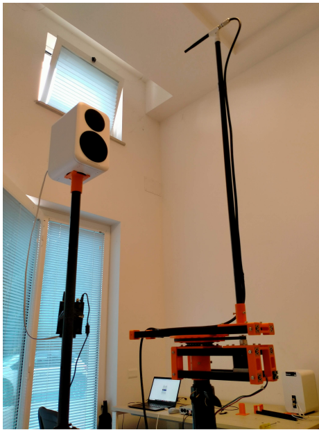
Fig. 5: Setup for polar measurement of a microphone.
