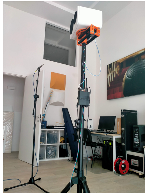
Fig. 3: Small two way loudspeaker measurement setup
