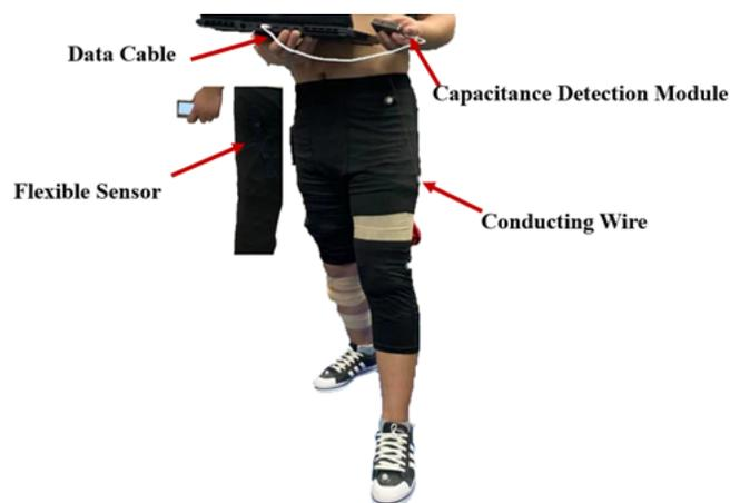
Fig. 1. Flexible stretchable sensor clothing for measuring the angle of lower limb joints, which is attached by Velcro to flexibly adjust the position.
