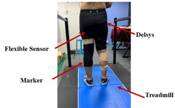
Fig. 6. Wearing sensor clothing to measure hip joint angle synchronously with Vicon on a treadmill.
