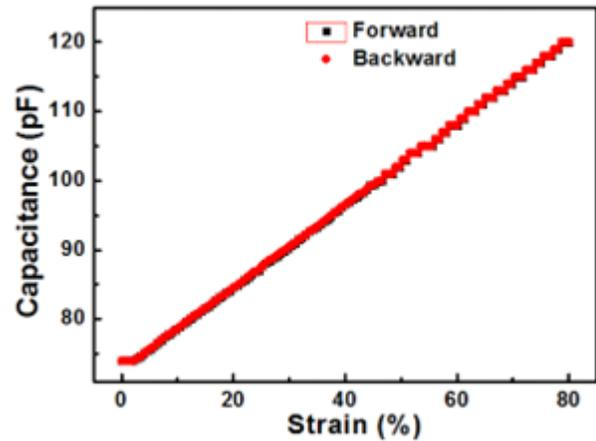
Fig. 4. The capacitance of the stretchable sensor as a function of the strain for a single stretch, showing high linearity and no hysteresis.
