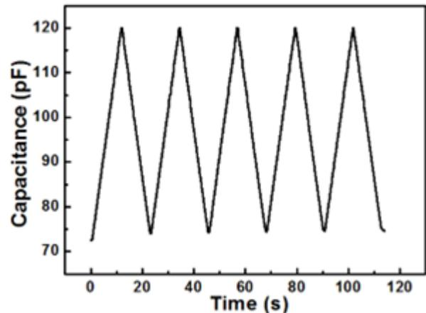
Fig. 5. The capacitance of the stretchable sensor as a function of the strain during extended cyclic tests.
