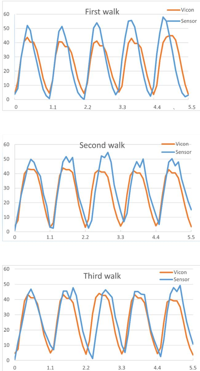
Fig. 7. Evaluating the synchronization of sensor clothing and Vicon. They are the angle time curves of the first three walks. Each walk has about five gaits, and each gait is 1.1 seconds.
