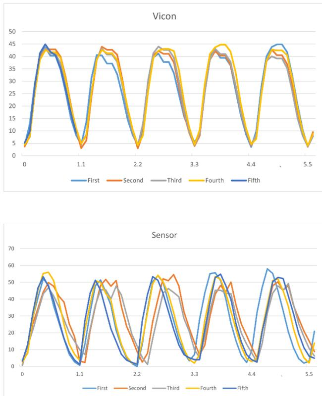
Fig. 8. Joint angle time curve of five walks of Vicon and sensor. The gait walking of Vicon and sensor were compared respectively.
