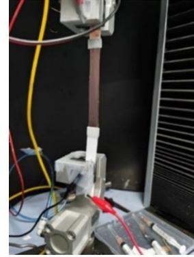
Fig. 3. The stretchable capacitance sensor being stretched by a mechanical
