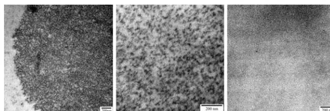
Figure 1. TEM micrographs of the PU/PBDO membranes containing (a) 10, (b) 25, and (c) 60 wt % PBDO [4].
