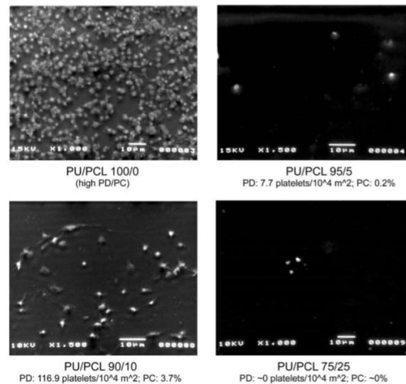
Figure 5. SEM microphotographs of the PU/PCL membranes after contact with platelets, and respective platelet deposition (PD) and platelet coverage (PC). In the PU/PCL 100/0 samples, quantitative image analysis could not be carried out due to the large degree of platelet aggregation[9].
