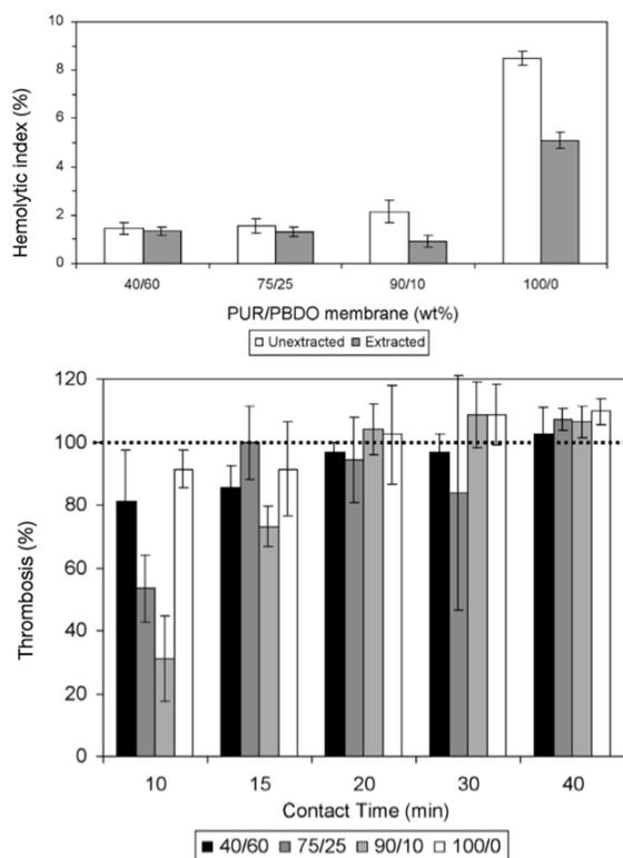
Figure 3. (a) Hemolytic index of the PU/PBDO membranes. (b) Percentage of thrombosis of the PU/PBDO membranes for different contact times with blood (glass: 100%, dotted line)[8].
