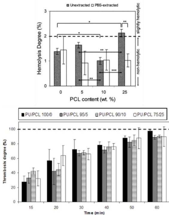
Figure 4. (a) Hemolytic index of the PU/PCL membranes. (b) Percentage of thrombosis of the PU/PCL membranes for different contact times with blood (glass: 100%, dotted line)[7].
