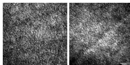
Figure 2. TEM micrographs of the PU/PDMS membranes containing (a) 25, (b) 75 wt % PDMS [8].
