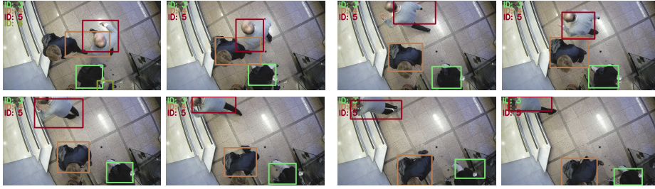
Fig. 4: Tracking sequence. The tracker attributes IDs and draws colored bounding boxes around the objects in every frame which it considers belong to the same object- each object has its own ID and color. The tracker is able to maintain these IDs even with multiple people going through the field of view. Here, four different IDs (from 2 to 5) are represented in different colors.
